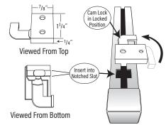
Slide Brackets into Notched Slot at top of track and evenly space them across the track. Use all brackets that are sent with the track.
