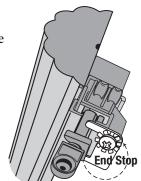
Remove any extra carriers and capture end most carrier with End Stop to lock remaining carriers within track. Tighten End Stop Screw to lock carriers in track.
